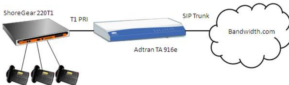
Figure A: ShoreTel's ShoreGear, Adtran's Total Access 916e connected with Bandwidth.com
